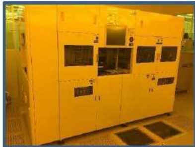
Thin Film Spin Coater
